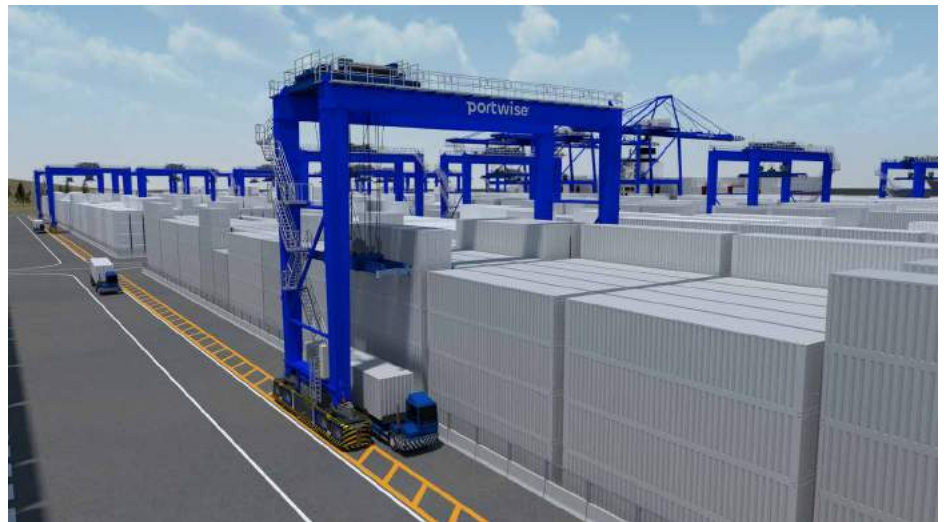
FIGURE 1. 3D image of an Automated Rubber Tyre Gantry crane, interchanging with a terminal truck.
