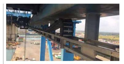
installed on their crane had small rollers that were integrated into the sideband links of the track at every metre. This design initially lowered the tow friction, but because only a very small portion of the roller was exposed over a relatively large gap, the wheels eventually failed turning this system into a gliding system.
