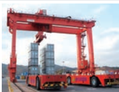
▲ Automated Transfer Crane and AGV for Kwangyang Port
