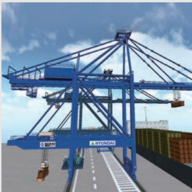
▲ Double Trolley Quay Crane with Automation System
