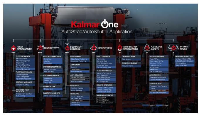
Each automated Kalmar One application has its own standardised blueprint. The dark blue modules are included in the Kalmar AutoStrad application by default, light blues are optional, and black modules are not applicable for AutoStrads at all.
