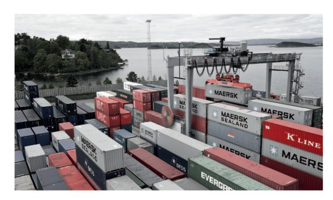
In a turnkey project, Kalmar is delivering eight revolutionary all-electric, 50-tonne RTGs, providing the Port of Oslo with the world's most sophisticated RTG installation that combines automated positioning technology and process automation. Semi-automation offers flexibility for the future, allowing the terminal to take automation to the next level when needed.
