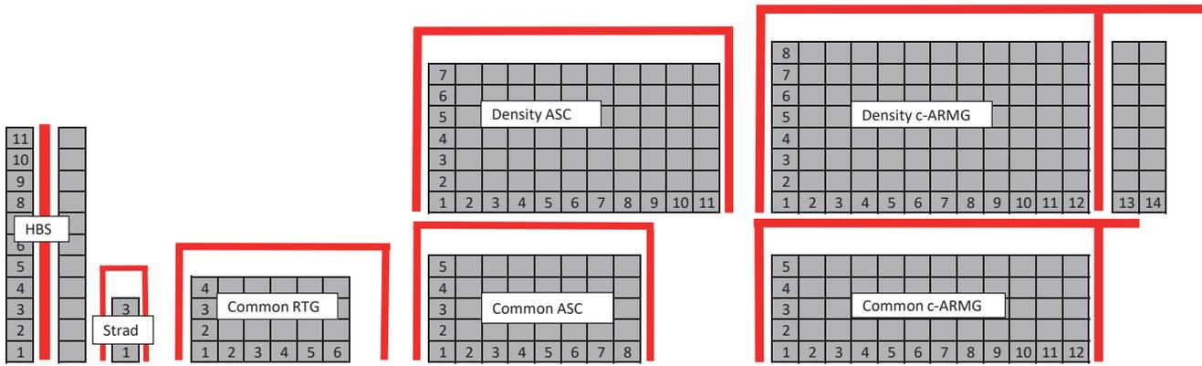
Figure 1: Stack Cross-Section of Yard Cranes
