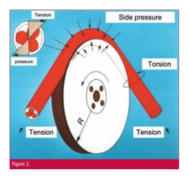
In the German standard DIN VDE 0298, the limit for pure tension is set much lower at 15N/mm (see dashed line named as  $\sigma$ -VDE). This seems very conservative and data sheets of several cable makers show that some allow more tension, for example 30N/mm<sup>2</sup>. This would seem acceptable as there is still room left within the elastic area. However, pure tension is not the only load on the copper.
