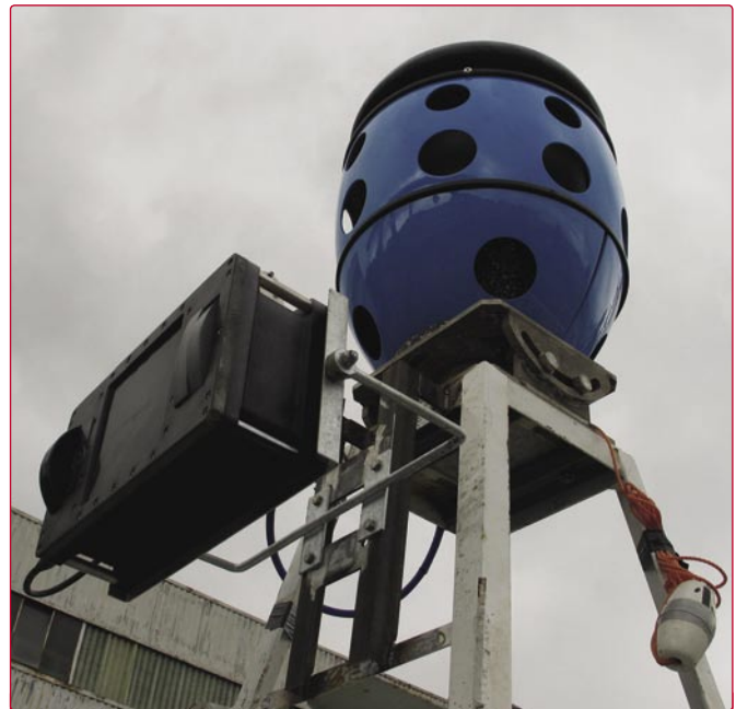
Figure 4. UK-based CodaOctopus' Echoscope sonar system was trialed in July 2005 with QinetiQ's Cerberus system as part of an integrated system for harbour protection to provide real-time, high-resolution visualisation of potential threats such as a diver entering a port zone.
