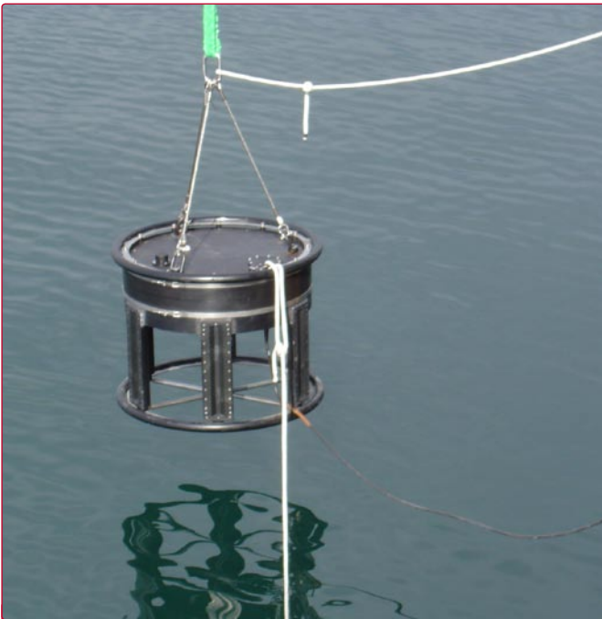
Figure 3. Lockheed Martin Canada's Swimmer Intruder Detection Harbour System is a 360°, long-range, high-frequency sonar designed to protect harbours and high-value coastal assets from underwater swimmer intruders.
