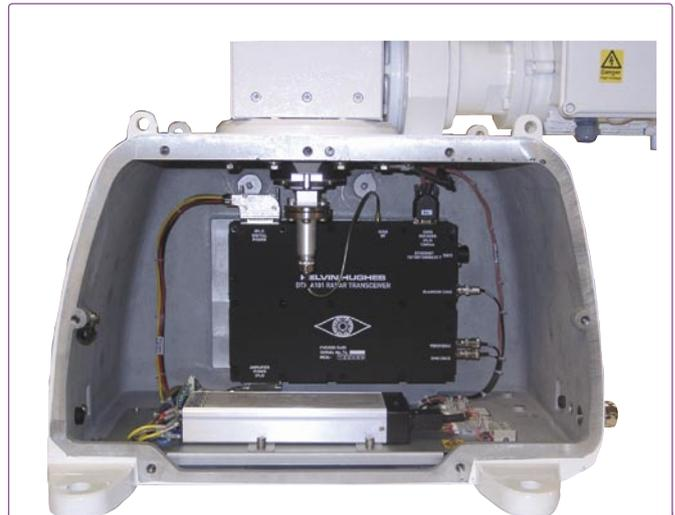
SHARPEye™ Upmast Transmitter configuration showing its compact nature with the power supply in the foreground and the transceiver mounted on the casing.
