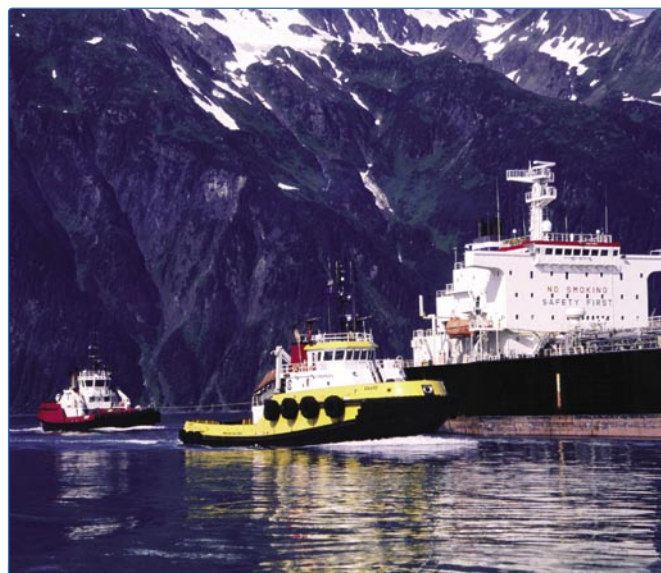
The Aware , a Crowley Azmuthing or Z-Drive tug, provides tanker assist and escort services through the Prince William Sound, Alaska to and from Valdez. The Z-Drive tug is best suited for ship assist and escort work in very narrow channels and harbours because of its superior bollard pull capabilities. The Tan'erliq , a Voith Schneider tug, is seen in the background.
