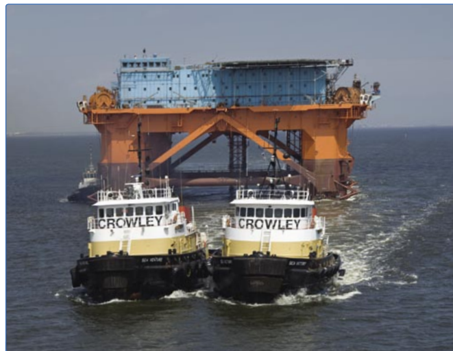
The Sea Victory and Sea Venture, both Crowley Invader-class, twin screw tugs, are shown towing of the Chemul, an ex-semi submersible drilling platform that is being converted as a floating hotel and work platform for PEMEX just outside the Port of Mobile in March 2008.
