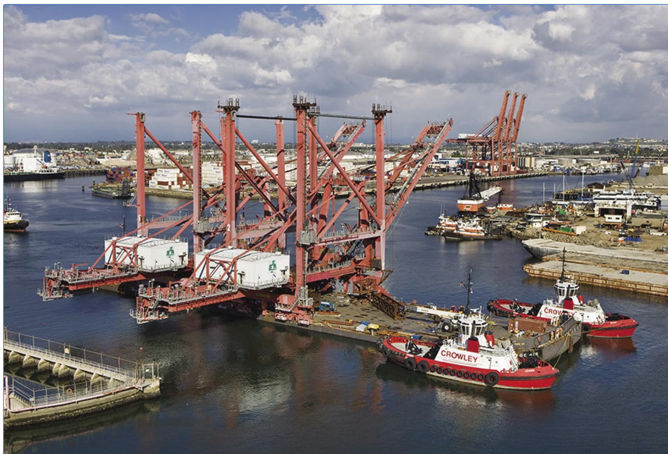
Crowley Voith Schneider tugs assist in the transport of cranes in the Port Los Angeles/Long Beach in November 2008. Voith Schneider tugs are equipped with a five-blade cycloidal propulsion system providing superior manoeuvrability essential for ship assist and escort operations, especially in tight areas.
