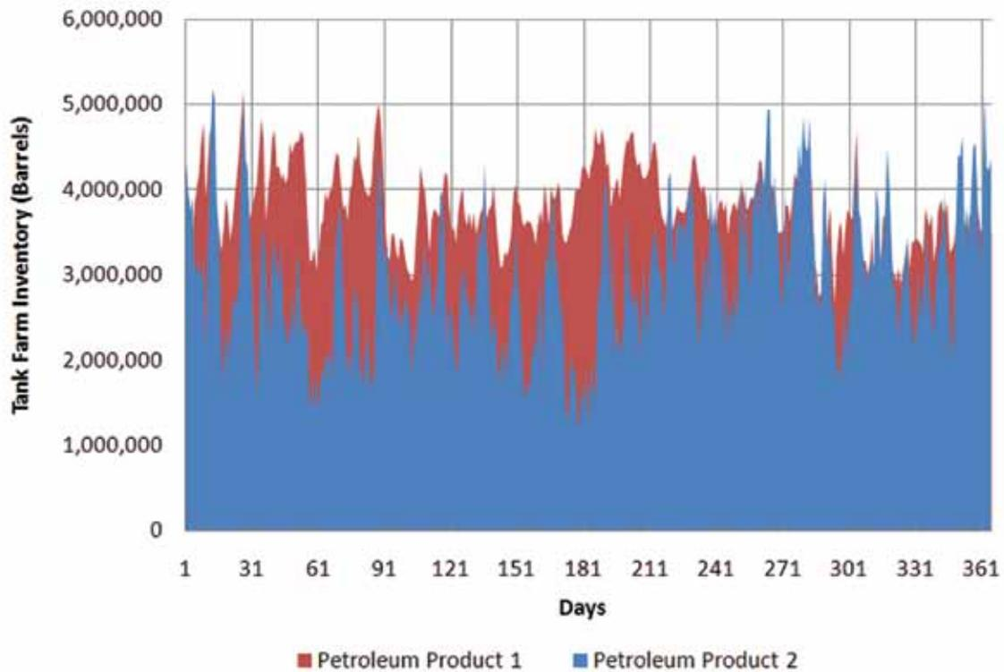
Figure 5. Simulation model output of tank farm inventory variation.
