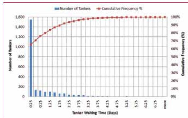
Figure 4. Sample simulation model output of tanker wait-time distribution.
