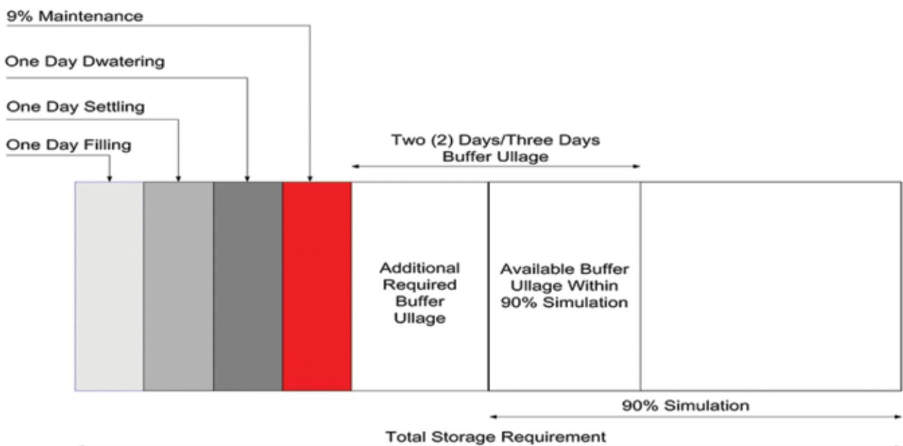
Figure 6. How simulated storage results can be used to determine total storage requirement.
