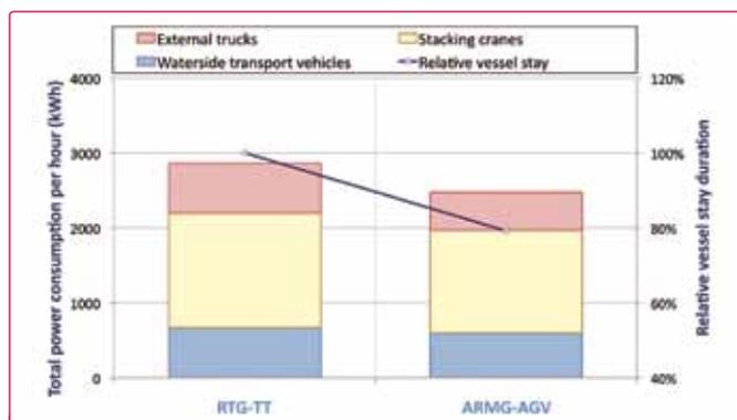
Figure 4. Power consumption during peak hour on RTG+TT terminal and ARMG+AGV terminal.
