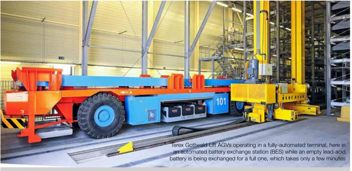
Terex Gottwald Lift AGVs operating in a fully-automated terminal, here in an automated battery exchange station (BES) while an empty lead-acid battery is being exchanged for a full one, which takes only a few minutes
