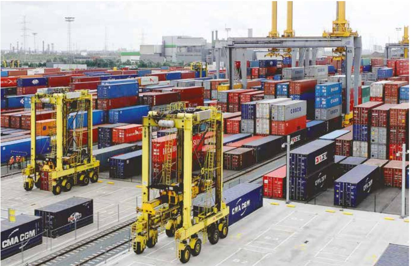
Manual Terex straddle carriers for horizontal container transport working hand in hand with Terex Gottwald automated stacking cranes
